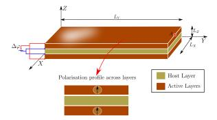
Bimorph piezoelectric polymer-based device, completely fixed at Y = 0, and subjected to  $\Delta \varphi = 10^4 \text{ V/m.}$  Symmetric boundary conditions have been applied at  $X_{med} = (\max(X) + \min(X))/2$ . Objective function aiming at maximising Z direction of displacement at point **A**. Polarisation profile across the thickness (vector **V** in equilibrium equations).
