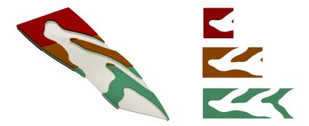
Design of the multilayered torsional piezoelectric actuator for  $p_m = 3$  and  $p_e = 6$ ,
