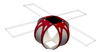
Dielectric elastomer-based gripper. Deformed configuration for voltage gradiens  $\Delta \varphi$  of  $(\frac{2}{3} \times 10^3) \times \{24\}$  V/m. Results obtained with the optimised design corresponding with  $p_m = 3$ ,  $p_e/p_m = 2$  using **continuation strategy**
