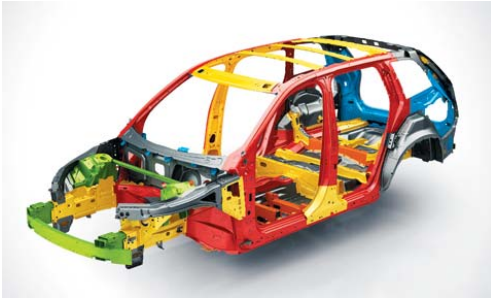
Volvo's 'XC90' chassis with various materials bonded together (from Volvo)
